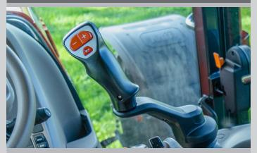
The multi-functional loader joystick is built with 3rd service and Powershift buttons, simplifying loader working conditions for the user.
