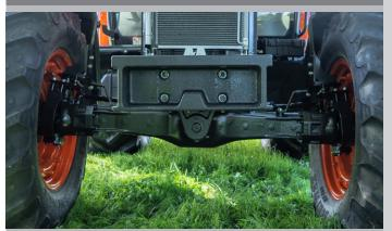
The use of a LSD front axle prevents the occurrence of slippage due to the load difference of the front wheels. This creates traction, greatly aiding manoeuvrability in any conditions.
