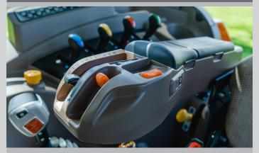
The multi-functional electronic armrest features numerous functions, such as throttle engagement, 3-point linkage lift and lower, Powershift and Auto Powershift mode.
