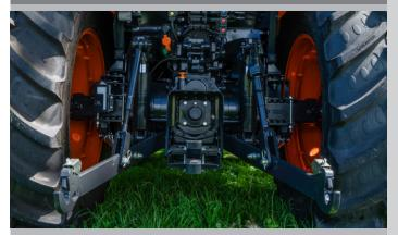
The electronic controlled 3-point linkage system boasts a 4852kg lifting capacity, allowing for the installation of multiple working implements.
