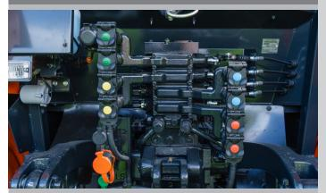
Load Sensing provides optimal hydraulic pressure and flow rate for load sensing operations. This results in automatically neutralising valves in the event of high loads during operation.
