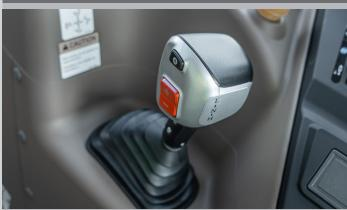
A simple button operation on the side speed lever and armrest gives you a 32x32 transmission with an 8-speed Powershift in 4 ranges.
