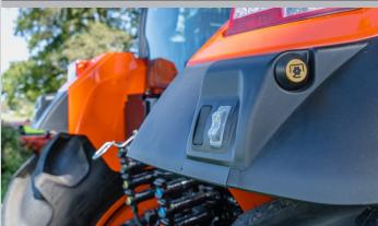
The addition of rear fender remote and PTO switches increases the convenience of both the removal and attachment of external implements.
